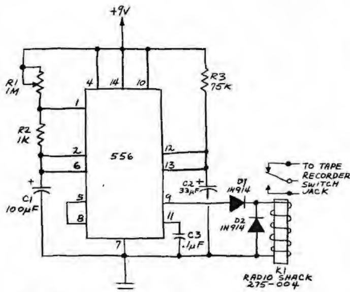
Fig. 4. This circuit, which employs a 556 dual timer, is functionally identical to the one shown in Fig. 3.
